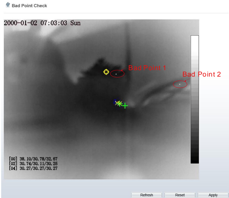
Figure 5-6 Bad point check interface
